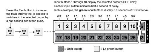
Figure 3-40 — Adjust the RGB delay interval
